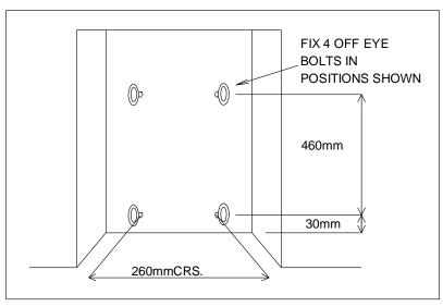
Fix the fire casing back into the opening using the cable fixing system as shown in do not cut off loose ends of cable after fixing, coil and tuck carefully behind sides of Refractory back Note: when using the cable fixing kit with the spacer, fix and seal the spacer to the rear of the appliance flange with the screws and foam seal provided.
